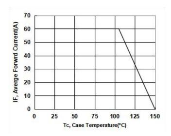
**Forward Current VS Case temperature Diode**
